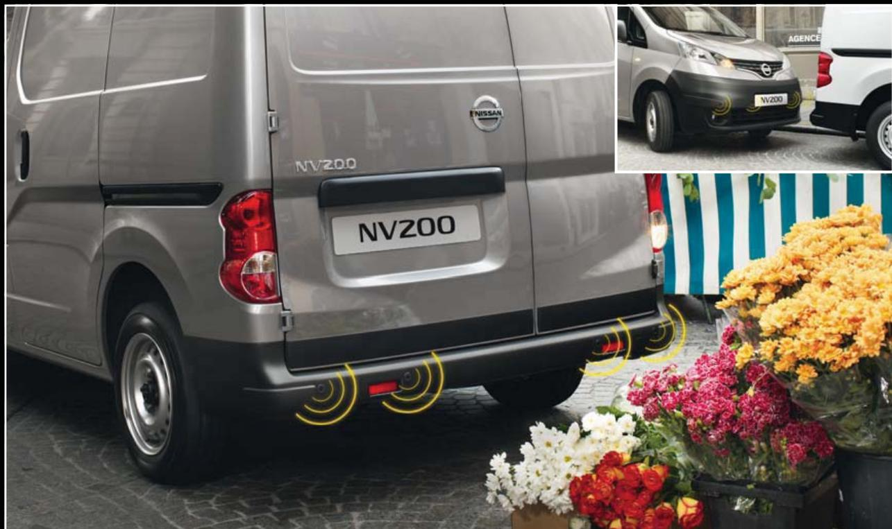
**The Rear Parking System**<sup>(29)</sup> sensors activate automatically when you engage reverse gear. An audible signal increases in frequency as you get closer to an obstacle, until a continuous tone warns you to stop\*. A Front Parking System<sup>(29)</sup> is also available. Door protection cladding is available to protect NV200's hatchback or French rear doors.
